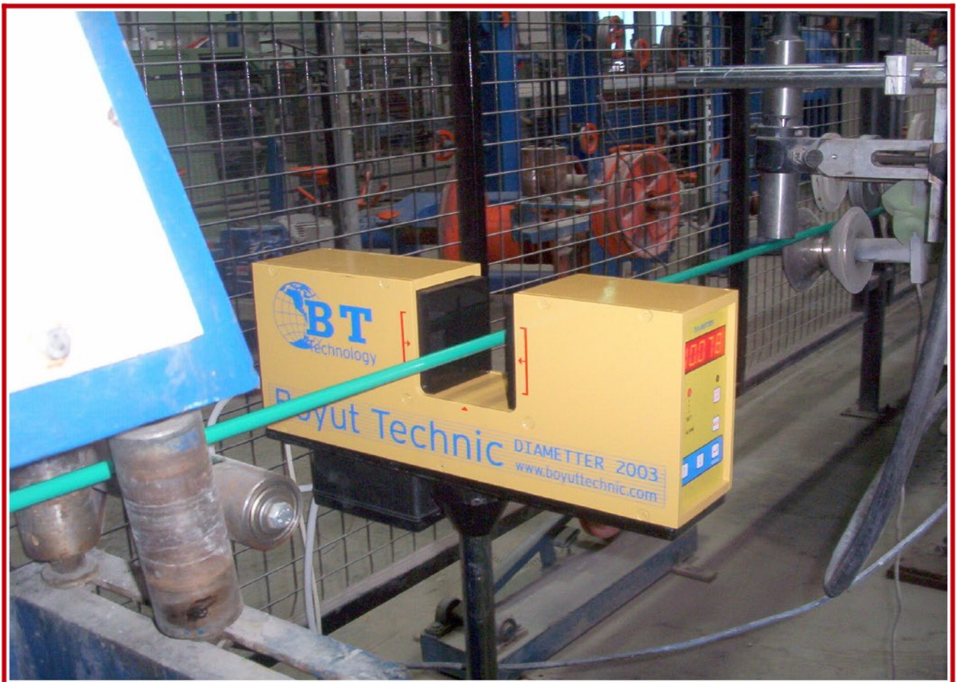
A SAMPLE APPLICATION of NON-CONTACT LASER MICROMETER at CABLE PRODUCTION LINE
